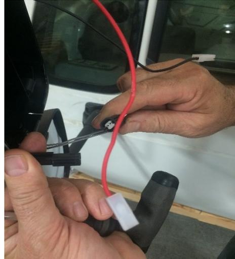
Figure 45: Wire Connector/Adapter Removal (motor)
