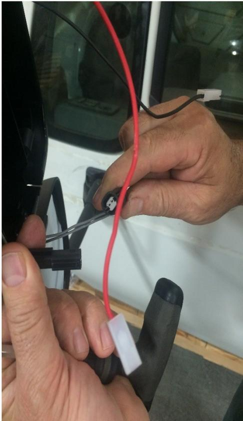
Figure 24: Wire Connector/Adapter Removal (w/o motor)
