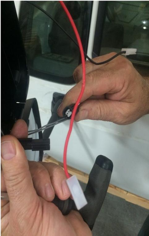
Figure 34: Wire Connector/Adapter Removal (w/o motor)
