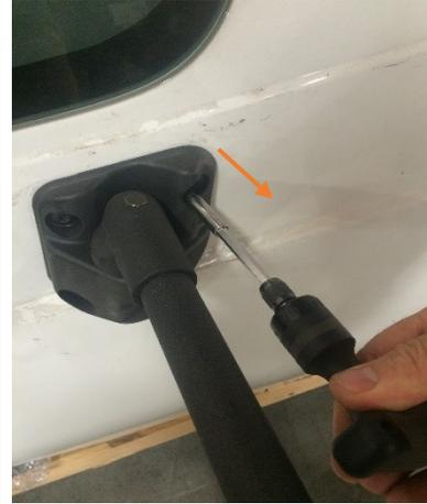
Figure 3: Bracket Removal (Lower Holder)
