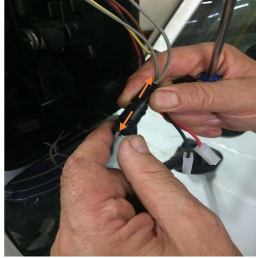
Figure 33: Wire Connector/Adapter Removal (w/o motor)
