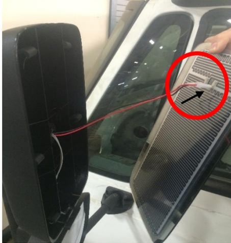
Figure 12: Main Glass Installation (Heater Wires)
