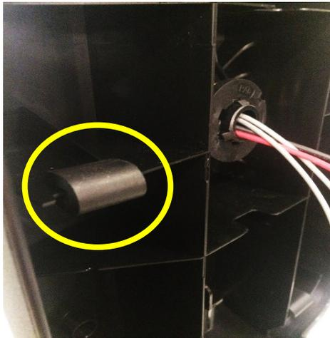
Figure 14: Main Glass Installation (Foam Pads)
