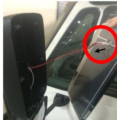
Figure 11: Main Glass Removal (Heater Wires)
