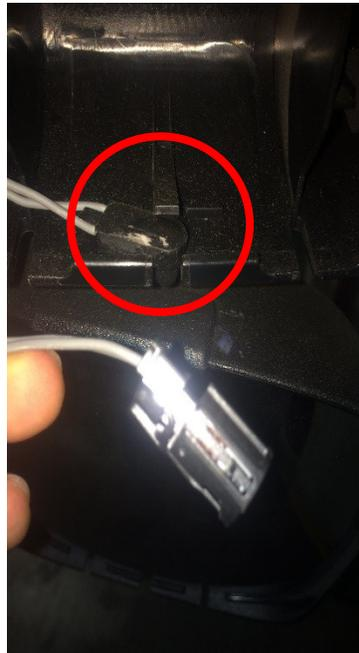
Figure 60: AAT Sensor Holding Clip
