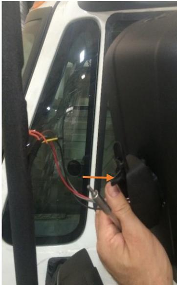
Figure 37: Convex Wire Installation (w/o motor)
