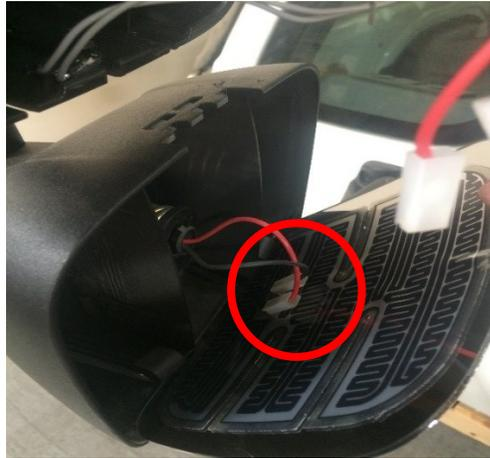
Figure 18: Convex Glass Removal (Heater Wires)
