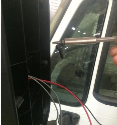
Figure 32: Convex Top Screw Removal (w/o motor)
