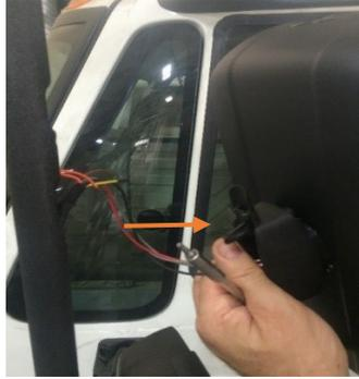
Figure 46: Wire Installation (motor)
