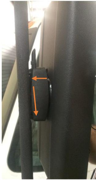
Figure 38: Convex Housing Installation (w/o motor)
