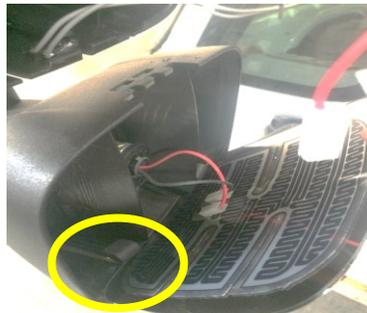
Figure 19: Convex Glass Installation (Foam Pads)
