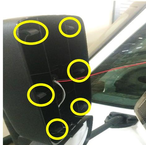
Figure 15: Main Glass Installation (Foam Pads)
