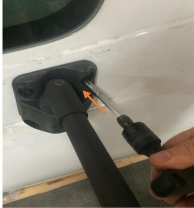
Figure 4: Bracket Installation (Lower Holder)
