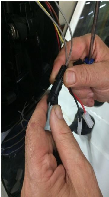
Figure 59: AAT Sensor Wire Connector
