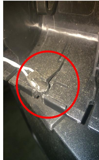
Figure 61: AAT Sensor Holding Clip
