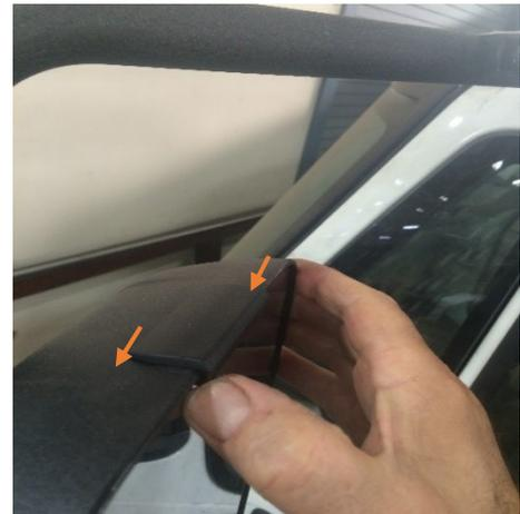
Figure 17: Main Glass Installation (Clip)
