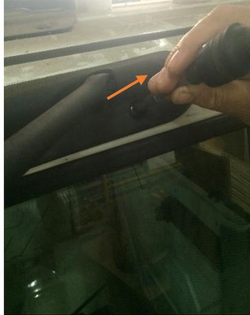
Figure 2: Bracket Removal (Upper Holder)
